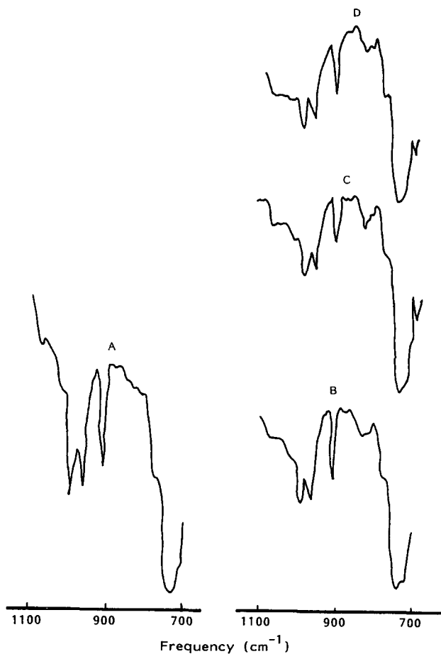
Figure 8 Infra-red spectra for polybutadiene and its cyclized products using the system \text{AlCl}_3/\text{CCl}_3\text{COOH} : (A) uncyclized; (B) \text{AlCl}_3 ( 9.7 \times 10^{-4} \text{ M} )/ \text{CCl}_3\text{COOH} ( 5.2 \times 10^{-3} \text{ M} ); (C) \text{AlCl}_3 ( 9.7 \times 10^{-4} \text{ M} )/ \text{CCl}_3\text{COOH} (0.01 M) and (D) \text{AlCl}_3 ( 9.7 \times 10^{-4} \text{ M} )/ \text{CCl}_3\text{COOH} ( 2 \times 10^{-3} \text{ M} )
